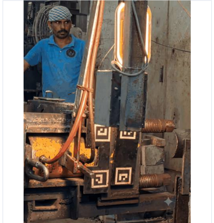
Camera view - four markers in frame. Vision device sees top and bottom markers on both plates during the pull.
